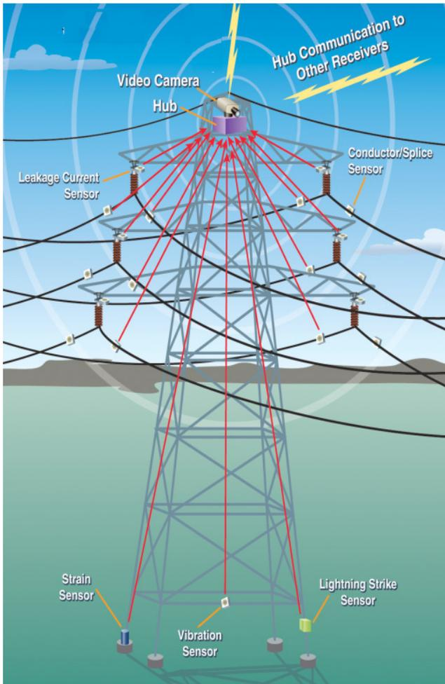
Figure 11. EPRI Transmission Line Wireless Sensor System
