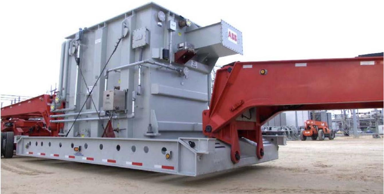
Figure 8. Recovery Transformer – (Photo Courtesy of DHS S&T)
