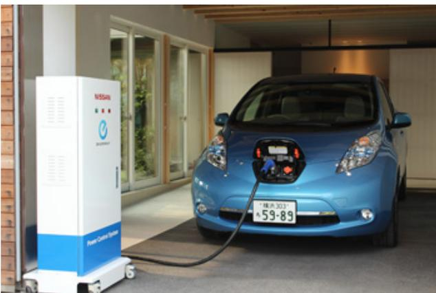
Figure 19. EV Power Source (Courtesy: Nissan) [77]
