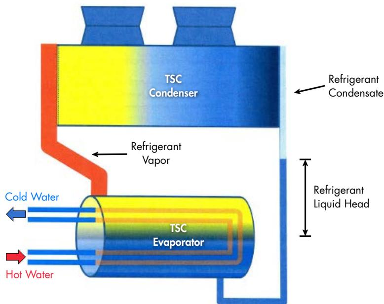
Figure 5. Flow Diagram for the TSC (figure used with permission from Johnson Controls)
