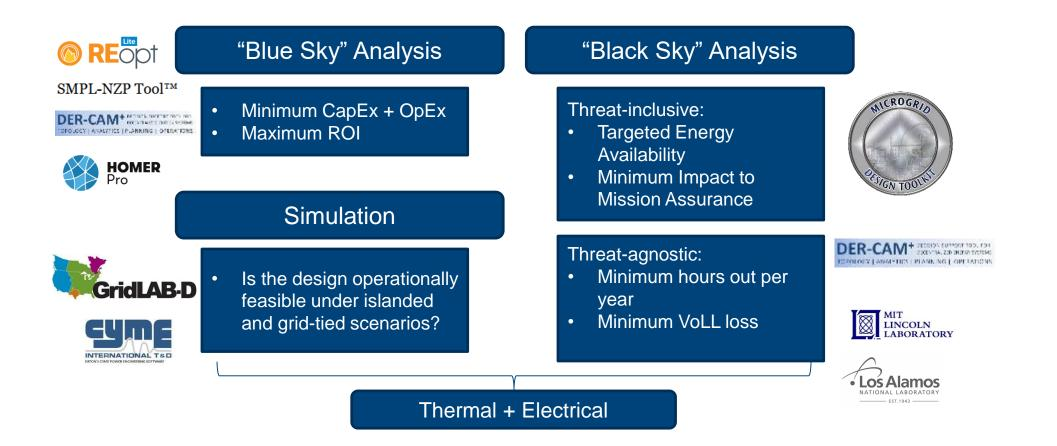
No single tool truly co-optimizes the microgrid design for **resilience + efficiency + sustainability** AND ensures the design is physically feasible/realistic
