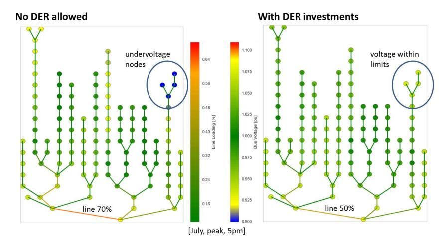
System-level visualization of grid impact on voltage levels, line loading
