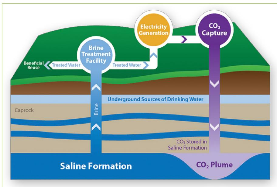
Carbon storage diagram showing CO<sub>2</sub> injection into a saline formation while producing brine for beneficial use.
